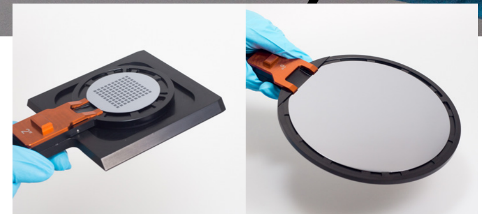
Top: Microlens arrays printed on a two-inch wafer substrate. Bottom left: Two-inch wafer substrate mounted on sample holder. Bottom right: Six-inch wafer substrate mounted on sample holder.
